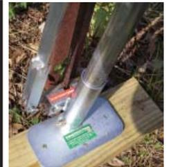
**Handle Extension:** Remove hitch pin in handle, extend inner handle to desired length and replace hitch pin. See below.
