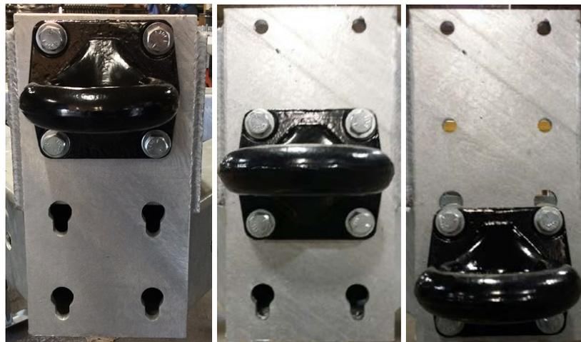
**Figure 6. Mounting Positions of Lunette Ring**
